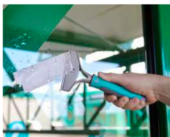
Blades designed to remove encrustations
