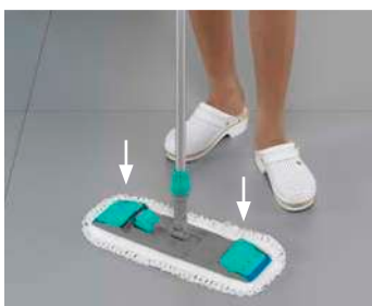
Press down the frame to close it
