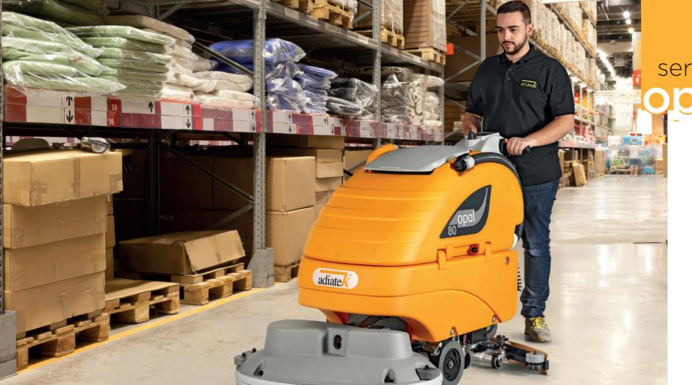
Equipped with a display and electronic controls, this model was designed for large areas. The brushes base is provided with two geared motors, one for each brush, and the suction motor can switch from standard to silent mode with just a click. It is also possible to equip this machine with both the Ozone and 3S systems.
