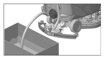
3. After the tank is completely drained, take off the drain box (1) by releasing the lever (2) and unscrew the cap (3).
