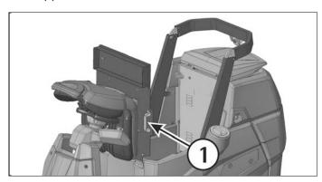
If the machine is equipped with the optional 3SD water system, it is necessary to take off the support of the detergent tanks after lifting the seat base.
