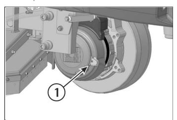
Release the machine from the wooden brackets by moving it backwards, as indicated in the figure, avoiding heavy contacts to mechanical parts.
