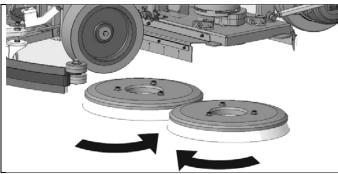
For a longer life of the brushes we suggest to invert daily their position. Whenever brushes result to be deformed we suggest reassembling them in the same position, in order to avoid that the different inclination of the bristles causes excessive motor overload or troublesome vibrations.
