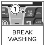
In this way automatically the brushes lift, the solenoid valve shuts down and it is possible to finish the drying operation for a total time of about 15 seconds, afterwards also the squeegee is lifted and the suction stops.
