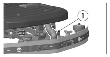
2. Wash the inside of the hose with a water jet.
