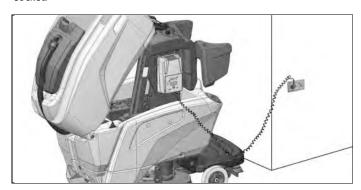
Never charge a GEL battery with a non suitable recharger. Strictly follow the instructions supplied by the batteries and recharger manufacturer NOTE: Never leave the batteries completely discharged for long periods even if the machine is not used. In case of traditional batteries, please check the electrolyte level every 20 recharging cycles and eventually fill them up with distilled water. Never leave the batteries discharged for more than two weeks.
