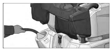
On the rear part of the machine is placed a level hose that permits to see easily the solution quantity inside the tank both during the filling of the solution and during the working.
