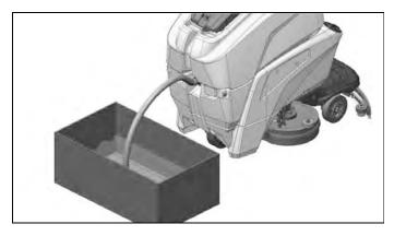
3. Clean the inside of the tank using a water jet.
