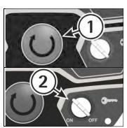
3. Use the key switch to turn off and then on the machine (2).
