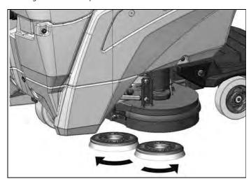
For a longer life of the brushes we suggest to invert daily their position. Whenever brushes result to be deformed we suggest reassembling them in the same position, in order to avoid that the different inclination of the bristles causes excessive motor overload or troublesome vibrations.
