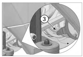
4. Move the machine backwards, as indicated in the figure, avoiding heavy contacts to mechanical parts.
