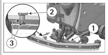
3. Block the squeegee by rotating the two knobs (2) clockwise. Insert the squeegee hose (4) into its coupling, respecting its 4. position as indicated in the figure.
