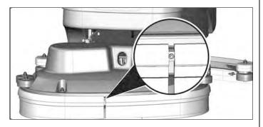
Screw down the knobs in the rear part of the cover in the free extremity of the metal strips. The operation has to be carried out for both splash guards. With the brushes assembled, the splash guard must slightly touch the floor.
