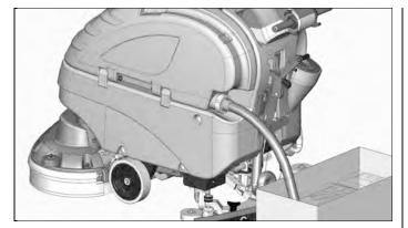
Open the cover of the recovery tank. 2. Rinse the tank with a water jet. 3.
