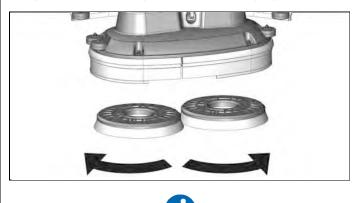
For a longer life of the brushes we suggest to invert daily their position. Whenever brushes were deformed we suggest to reassemble them in the same position, avoiding that the different inclination of the bristles causes excessive motor overload or troublesome vibrations.
