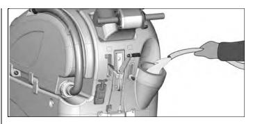
Always on the left side of the machine there is placed a level hose that permits to see easily the solution quantity inside the tank both during the filling of the solution and during the working.
