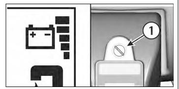
Check that the battery connector is correctly plugged in.
