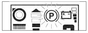
This control blocks the machine immediately stopping all functions. The emergency brake functions also as a parking brake. To start again to work, release the lever by unblocking the parking button on the lever itself and act again upon the levers drive control.
