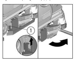
6. Take off the stop (2) then unscrew and take off the knob so to open the blocking support as shown in the figure.
