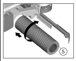
10. During the reassembly of the brush (6), insert it into the brush base from the part where the seat is deeper (about 40mm). The opposite part with a depth of about 13,5mm has to look towards the support plate.
