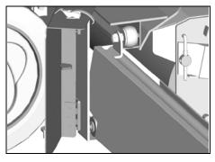
10. Close the door (2) and reposition the bar of the side rubber.
