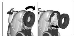
To reassemble the brush, insert the coupling buttons into the slots of the brush holder plate and rotate counterclockwise until it locks.
