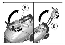
To avoid excessive stress on the handle bar it is recommended to empty the solution tank (see under "EMPTYING AND CLEANING OF THE SOLUTION TANK") if you were to cover very uneven flooring (eg. asphalt or cobblestones).
