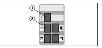
If the machine is equipped with a display, on the display (1) the following indication of the battery charge level is digital and indicates the percentage of the battery charge. 100 is the maximum charge, down to a minimum of 10, indicating every 10% decrease. When the charge level reaches 20%, the display starts blinking indicating the end of the battery charge.
