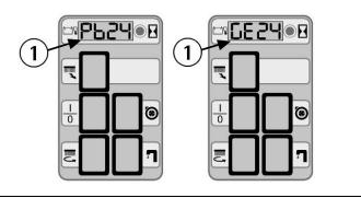
In case of GEL batteries installation, it is necessary to carry out a specific adjustment. Please contact the authorized technical assistance.
