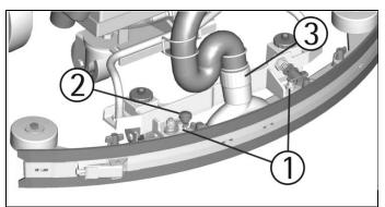
3. Uncouple the hook (1) of the rubber holder blade, release the extremities (2) from the squeegee body and take off the rubber (4).
