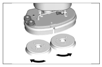
To unlock the brush, perform the same operations and rotate the brush the opposite way as for the locking.
