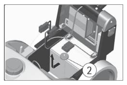
5. Take off the other battery (4) making it slide forwards in the battery compartment, then take it off.
